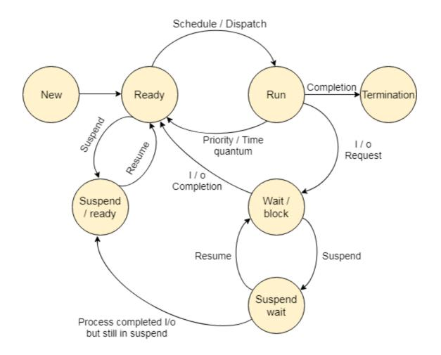
The process, from its creation to completion, passes through various states. The minimum number of states is five.
